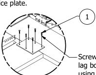
Screw in (6) 14-10 lag bolts into each splice plate using a #3 square drive.
