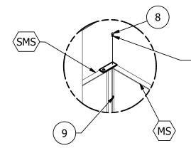
Secure main screen to side screen with (1) 1/4-20 bolt using a 5/32 Hex Drive. Secure bolt with (1) 1/4-20 nut using a 7/16 Crescent Wrench.
