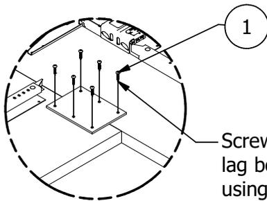
Screw in (6) 14-10 lag bolts into each splice plate using a #3 square drive.
