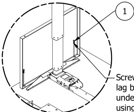
Screw in (2) 14-10 lag bolts into screen on the underside of the top using a #3 square drive.
