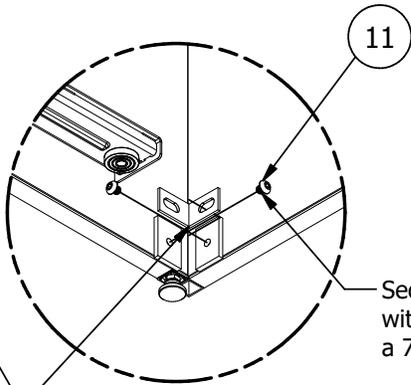
Secure main shell to side shell with angle bracket and (2) 3/8-16x3/8 bolts using a 7/32 Hex Drive at the top and bottom of joint.
