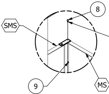
Secure main screen to side screen with (1) 1/4-20 bolt using a 5/32 Hex Drive. Secure bolt with (1) 1/4-20 nut using a 7/16 Crescent Wrench.
