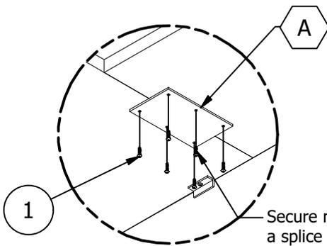
Secure main top and return top together with a splice plate at connection and lag bolts.
