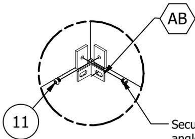
Secure main shell to side shell with angle bracket and (2) 3/8-16x3/8 bolts using a 7/32 hex drive at the top and bottom of joint.
