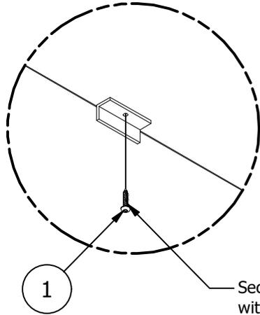
Secure main top to assembled shell with lag bolts using a #3 square drive.
