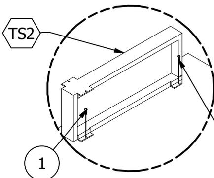
Secure transaction screen to main top with lag bolts using a #3 square drive.
