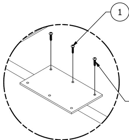
Attach splice plate at connection with (3) 14-10 lag bolts using a #3 square drive.
