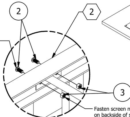
Fasten screen nut to screen bolt on backside of screen using a 15/16 crescent wrench.
