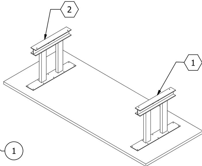
Screw in (10) 14-10 Lag bolts in each leg using a #3 square drive.
