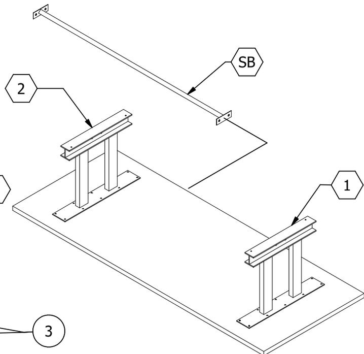
Insert screen bolts into the support bar through the tabbed legs using a 3/8 hex drive.
