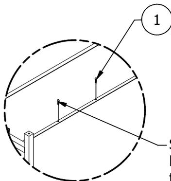
Screw in (5) 14-10 lag bolts into screen on the bottom of top.
