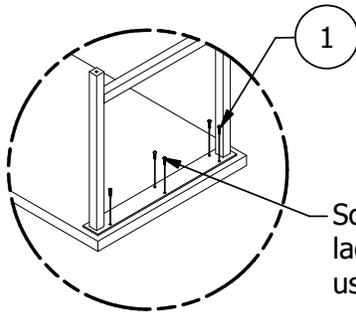
Screw in (6) 14-10 lag bolts in each leg using a #3 square drive.
